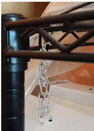
Figure 2. Use of light-duty chain and S-hooks to adjust the height of the fluorescent lamp (photo credit: Whitt Environmental Services)
