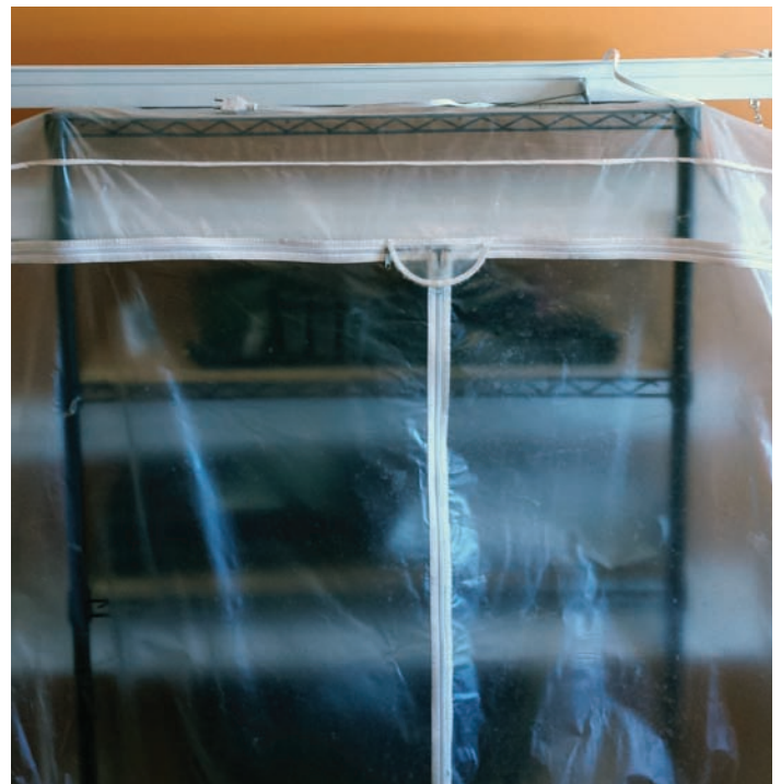
Figure 1. Use of a repurposed plastic wardrobe cover as a plant growth test enclosure (photo credit: Whitt Environmental Services)
